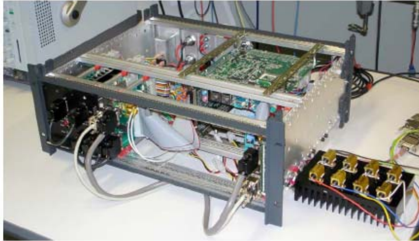
Figure 46: The prototype control electronics rack during bench tests. This unit will be mounted with the MOSFIRE electronics at the rear of the instrument.
