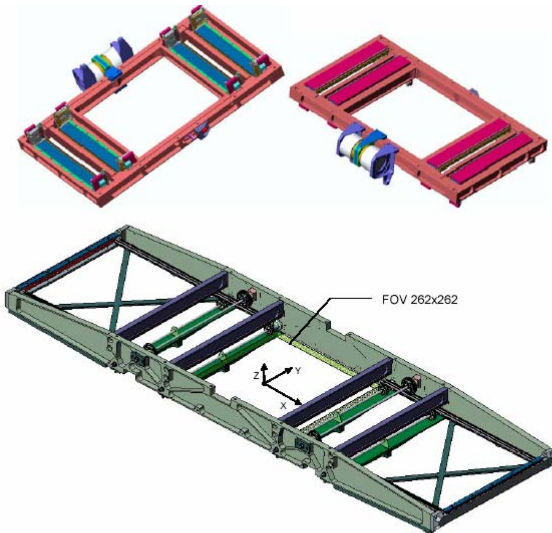
Figure 39: Two major CSU sub-assemblies: the Indexing Stage (top) and Support Frame (bottom)
