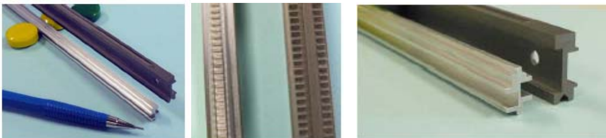
Figure 42: The new EUX bar (bare aluminum) alongside the previous larger bar (darker finish) developed for JWST. The rightmost pictures show the bar profile and drive grooves.
